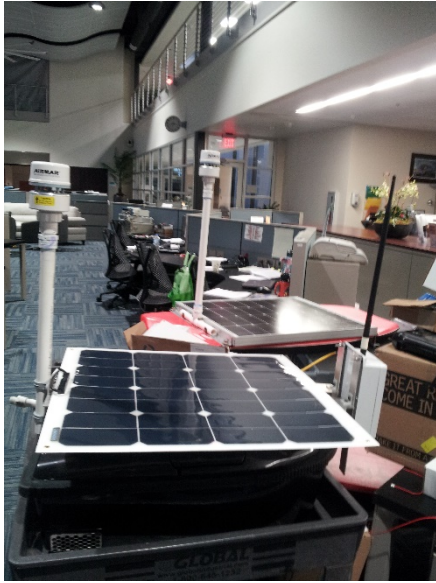
Version 1: Using bait boat structure, flexible solar panel and small 12V motor propulsion
